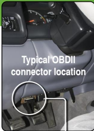
Typical OBDII connector location
